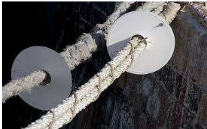
Fig. 6. Guard around cables and ropes
