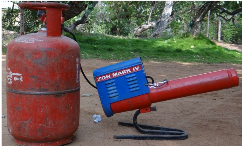
(b) Automatic mechanical bird scarer or pyrotechnic method
