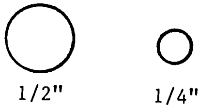
Fig. 2. Rats can given entry through holes as small as 1/2 inch (1.3 cm) in diameter, mice can get through a hole 1/4 inch (6.5 mm) in diameter.
